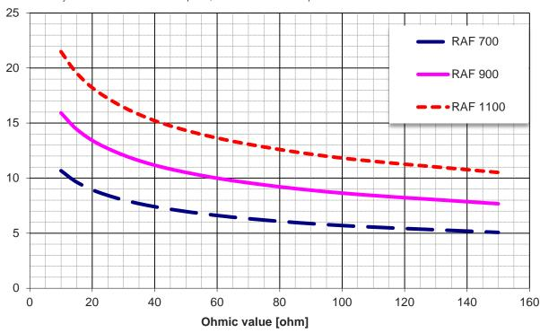
The rater power stated in this datasheet refers to the resistor mounted in horizontal position at the ambient temperature of 25°C and 250°C on the external surface. The power dissipation is influenced by:
