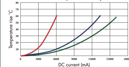
1. All test data is referenced to 25°C ambient.
