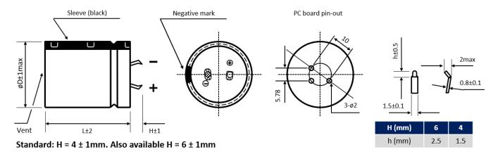
Multipin version ■ Diameter ø D ≥ 30 mm
