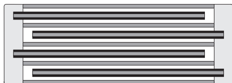
Extended double side metallized carrier film design
