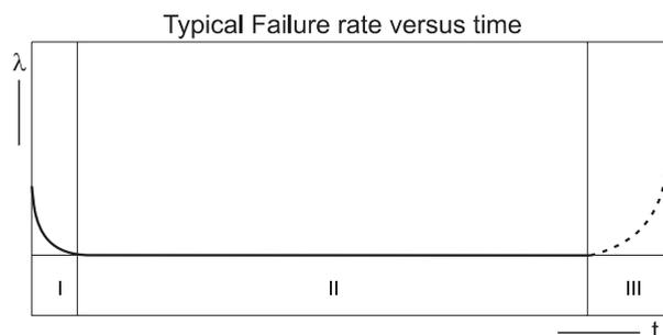
**Failure rates data at specifications are typically referred to the second period (II) only.**
