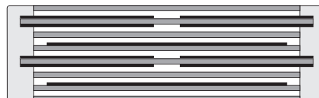
Extended double side metallized carrier film design with internal series connection and metallized film (series connection of 2 elements)
