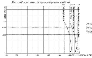
Curve a: DCB, PHC, RHB, RMC, PPS, PPA, RSB, RMB, MAR. Curve b: other series for power applications. Always refer to the max. operating temperature at specifications.
