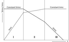
I: area where voltage is limited by ionization II: area where voltage and current are limited by reactive power dissipation and tg $\delta$ III: area where current is limited by terminals characteristics
