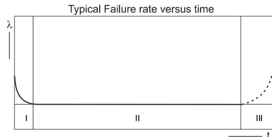
Failure rates data at specifications are typically referred to the second period (II).
