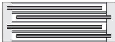
Extended double side metallized carrier film design
