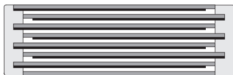
Extended metallized film design
