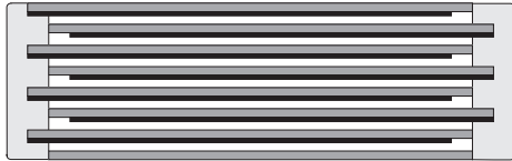
Extended metallized film design
